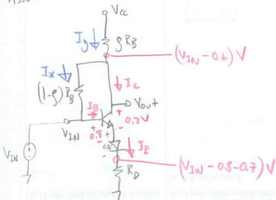
$$I_X = \frac{(V_{IN} - 0.6) - V_{IN}}{(1-g)R_B} = -\frac{0.6}{(1-g)R_B} A \quad ; \quad I_y = \frac{V_{CC} - (V_{IN} - 0.6)}{gR_B}$$
