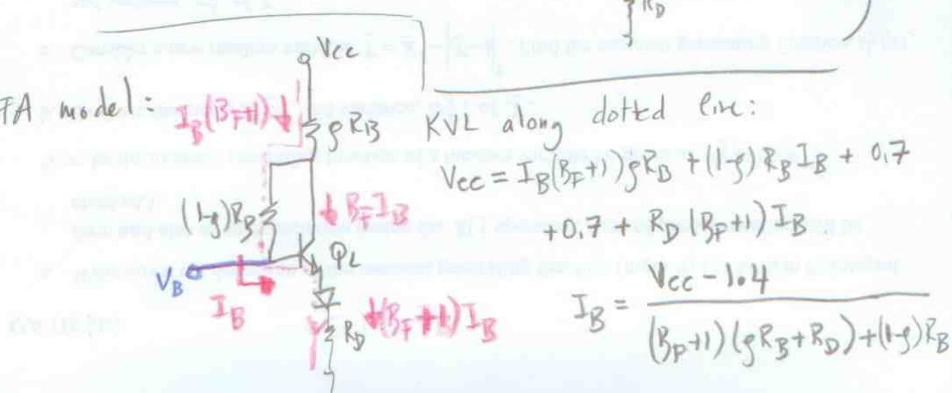
Using 93D Series Parameters ( $B_F = 100$ )
