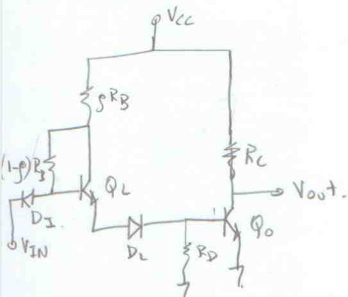
DTL with the following parameters is manufactured as 930 Series.
