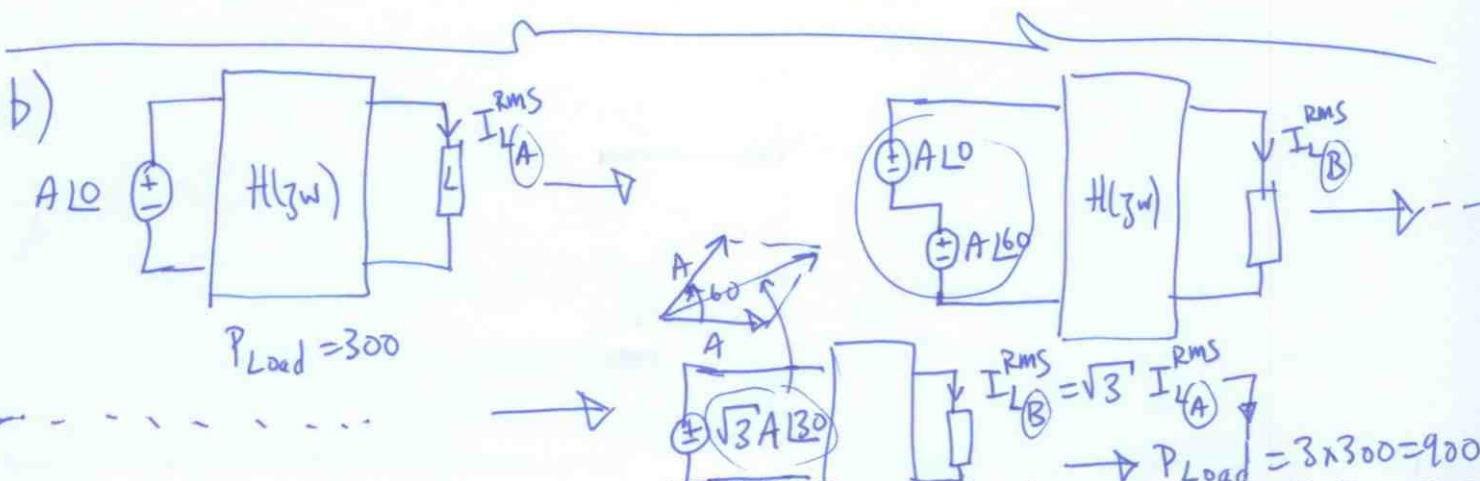
Question 2 (24 pts) Consider the following balanced three-phase circuit with  $\Delta$ -connected inductive load.
