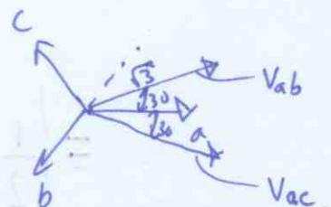
$$\begin{aligned} WM_2 &\Rightarrow Re \left\{ \sqrt{3} V_{ph}^{RMS} [130] I_{ph}^{RMS} [1 - \theta_L] \right\} \\ &= \sqrt{3} V_{ph}^{RMS} I_{ph}^{RMS} \cos(-30 + \theta_L) \\ &= \frac{1500}{2} + \frac{500\sqrt{3}}{\sqrt{3} \cdot 2} = 1000 \text{ Watt.} \end{aligned}$$
