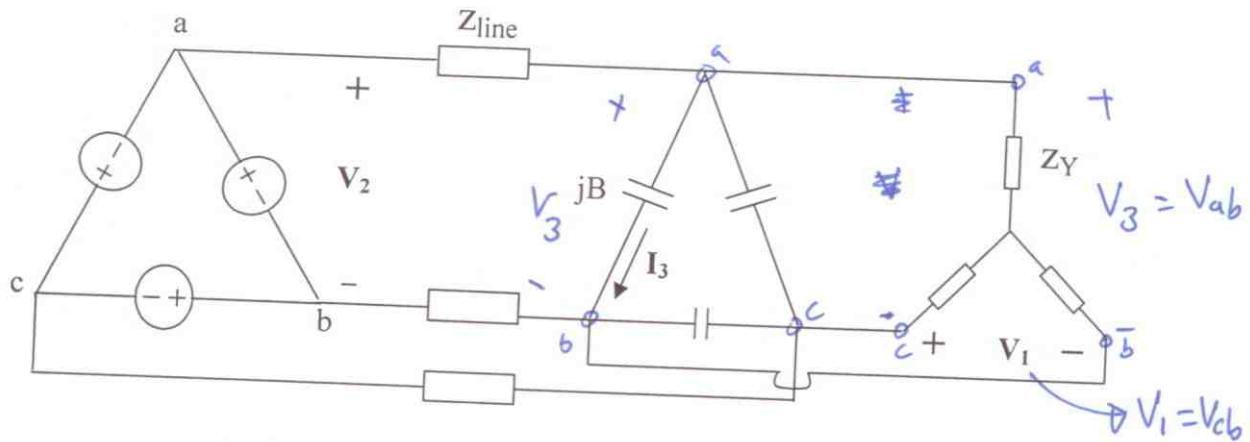
$$f = 50 \text{ Hz}, \quad Z_{\text{line}} = 0.4 + j1.2 \Omega, \quad Y_Y = \frac{2}{9} - j\frac{1}{6} \text{ mhos}$$
