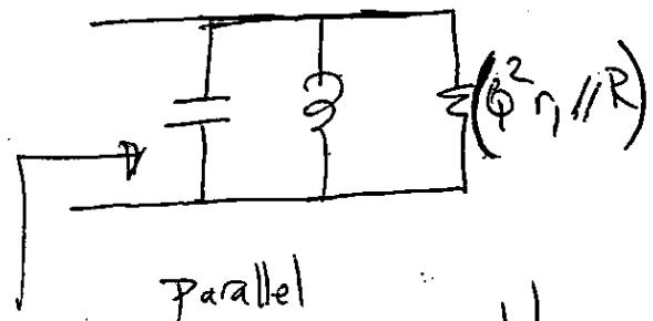
Parallel Standard resonance circuit!
