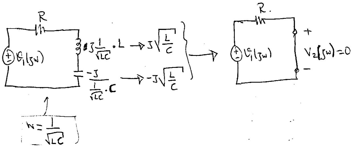
Note that  $V_1(j\omega)$  source sees purely resistive circuit at  $\omega = \frac{1}{\sqrt{LC}}$
