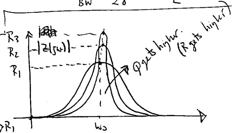
The maximum impedance is seen at resonance freq.
