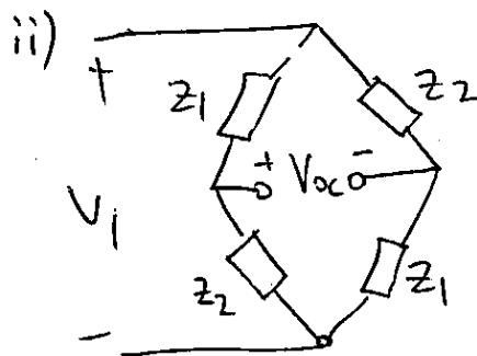
$$V_{oc} = V_1 \left( \frac{z_2 - z_1}{z_1 + z_2} \right)$$
