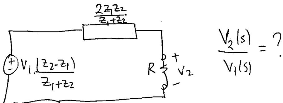
$$\frac{V_2(s)}{V_1(s)} = \frac{(z_2 - z_1)}{z_1 + z_2} \cdot \frac{R}{R + \frac{2z_1 z_2}{z_1 + z_2}} = (z_2 - z_1) \cdot \frac{R}{R(z_1 + z_2) + 2z_1 z_2}$$
