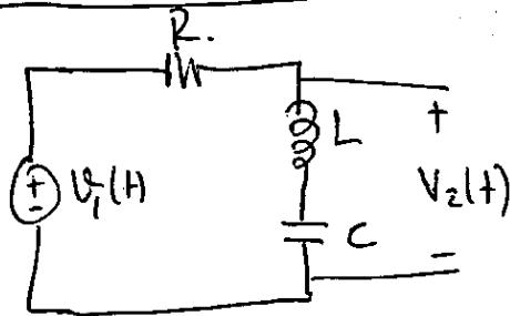
$$H(s) = \frac{V_2(s)}{V_1(s)} = \frac{sL + \frac{1}{sC}}{sL + \frac{1}{sC} + R}$$
