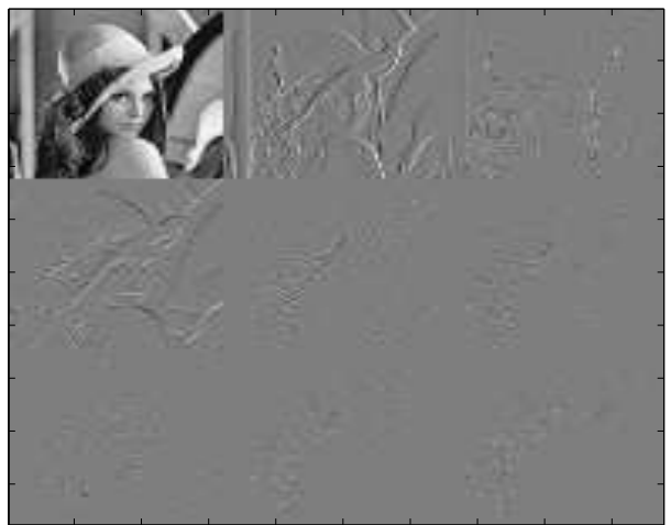
Fig. 1. DCT Channels: Collection of the same indexed DCT coefficients. The DC channel and eight other low frequency channels are illustrated for Lena image.
